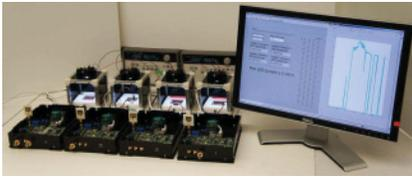
Fig. 3. A software-based light control system, along with four EnHANT prototypes.
