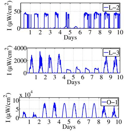
Fig. 5. Sample irradiance measurements in locations L-2, L-3, and O-1 (Mar. 2, 2010 - Mar. 12, 2010).
