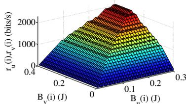
Fig. 14. Optimal communication rates  $r_u(i)$  and  $r_v(i)$  for different energy storage states, obtained by solving the *LSPD* problem for linear storage.
