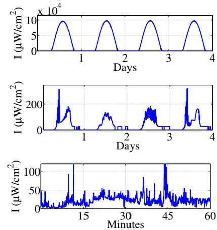
Fig. 1. Examples of different light energy sources: (top) *predictable profile* (Las Vegas, NV [5], outdoors), (middle) *partially-predictable profile* (New York, NY, a static indoor device), and (bottom) *stochastic behavior* (New York, NY, a mobile device in Times Square at nighttime).
