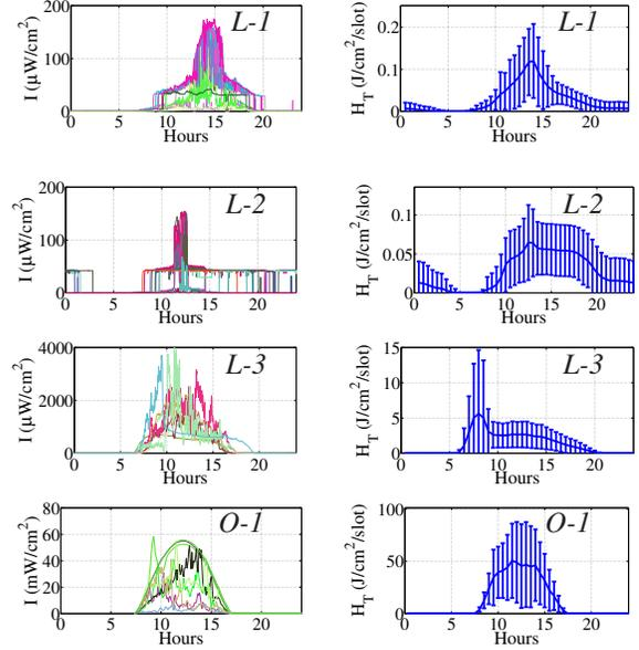
Fig. 7. Sample *energy profiles* for indoor locations  $L-1$ ,  $L-2$ ,  $L-3$ , and for the outdoor installation  $O-1$ . Left: irradiance measurements from several different days, overlaid; Right:  $\overline{H}_T$  values, with errorbars representing  $\sigma(H_T)$ .
