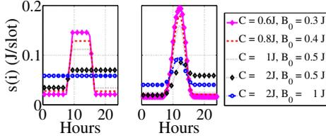
Fig. 11. Energy spending rates  $s(i)$ : obtained by solving the *TFLA-LIN* and *TFU-LIN* problems (left), and by solving the *TFU* problem for *nonlinear storage* (right).
