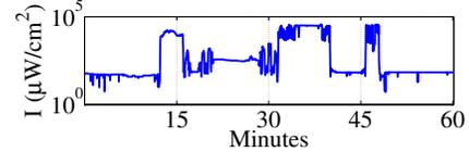
Fig. 10. Irradiance measurements recorded by a mobile device: a mix of indoor and outdoor conditions (note the log scale of the  $y$ -axis).
