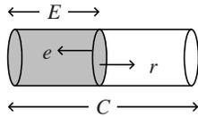
**Figure 3: An abstraction of an energy harvesting system for the upper layers: the energy storage capacity  $C$ , the current energy level  $E$ , the energy charge rate  $r$ , and the energy consumption rate  $e$ .**
