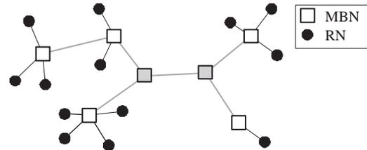
**Figure 1: A Mobile Backbone Network in which every Regular Node (RN) can directly communicate with at least one Mobile Backbone Node (MBN). All communication is routed through a connected network formed by the MBNs.**
