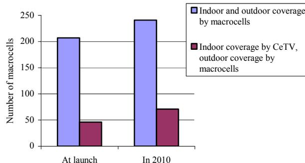
Figure 13. The number of macrocells in a UMTS network with and without CeTV deployment
