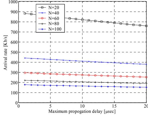
Figure 9. The arrival rate (to the access point of frames destined to a single station) in which the load is 0.8 as a function of the maximum propagation delay. The system is operated according to the VPP, with  $p_s^d = 0.3$ ,  $p_s^u = 0.9$ , and  $g = 1.2$
