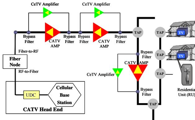
Figure 2. The CeTV system architecture
