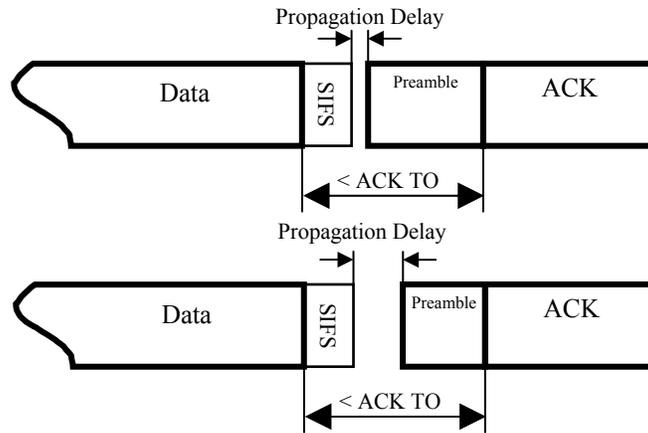
Figure 14. Using a short preamble in order to allow for a long propagation delay
