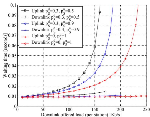
Figure 6. The mean waiting time (in the uplink and downlink queues) in a system operated according to the VPP as a function of the downlink offered load (per station). The number of stations is 100 and  $g = 1.2$
