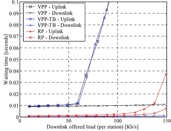
Figure 12. The average waiting time computed via simulation in systems operated according to VPP, VPP-TB, and RP. The arrival process is On/Off, the number of stations is 100,  $p_s^d = 0.3$ ,  $p_s^u = 0.9$ , and  $g = 1.2$
