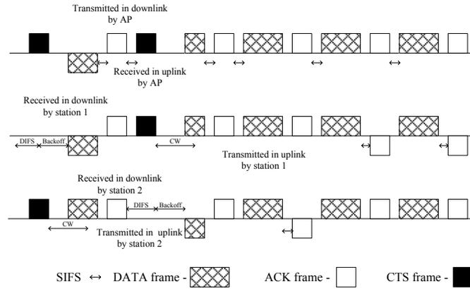
Figure 4. An example of the operation of the Virtual Polling Protocol in a network with an access point and 2 stations
