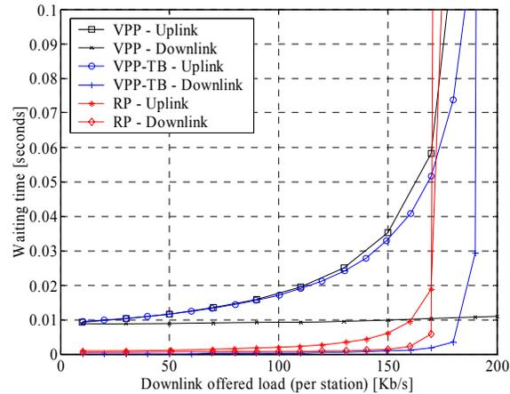
Figure 11. The average waiting time computed via simulation in systems operated according to VPP, VPP-TB, and RP. The arrival process is Poisson, the number of stations is 100,  $p_s^d = 0.3$ ,  $p_s^u = 0.9$ , and  $g = 1.2$
