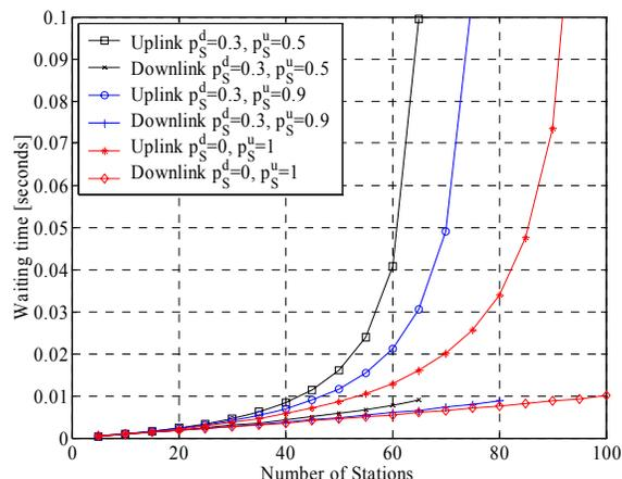
Figure 7. The mean waiting time in a system operated according to the VPP as a function of the number of stations. The arrival rate to the access point of frames destined to a single station is 256Kb/s and  $g = 1.2$
