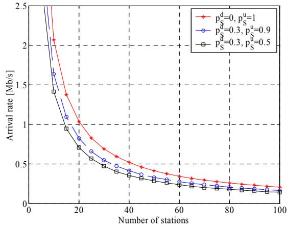
Figure 8. The arrival rate (to the access point of frames destined to a single station) in which the load is 0.8. The system is operated according to the VPP and  $g = 1.2$
