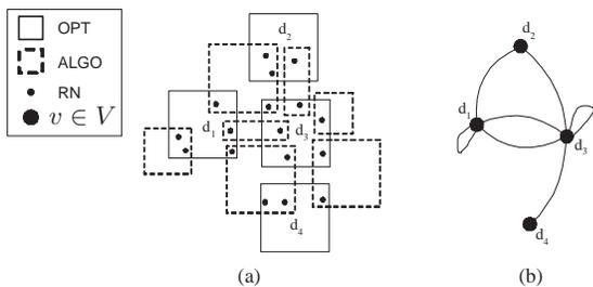
Fig. 4. Demonstration of a graph transformation: (a) original network and square cover, and (b) transformed graph.
