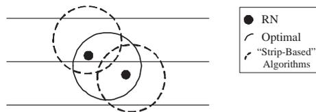
Fig. 2. Example of basic inefficiency of strip-based algorithms.
