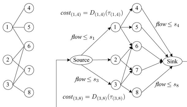
**Fig. 3** An example of the transformation of a bipartite graph to a flow network
