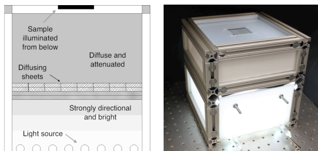
Figure 3 Indoor lighting simulator cross-section (left) and photo (right). PV cell is placed at the top center. Note the visible attenuation and uniformity at the top surface.
