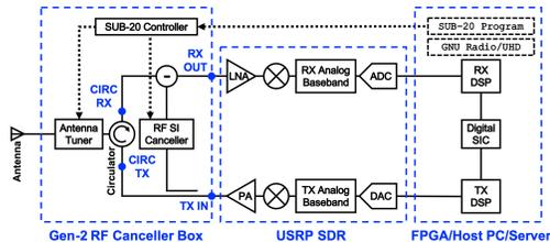
Fig. 1: Block diagram of the implemented Gen-2 wideband full-duplex (FD) radio consisting of a Gen-2 RF canceller box, a USRP software-defined radio (SDR), and a compute node (e.g., a host PC/server).
