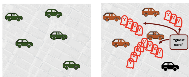
(a) Actual state of the road. (b) Reflected state (jammed) due to the attack.
