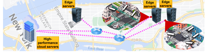
Figure 1: The NSF COSMOS testbed provides cameras and edge servers for piloting real-time video analytics systems.
